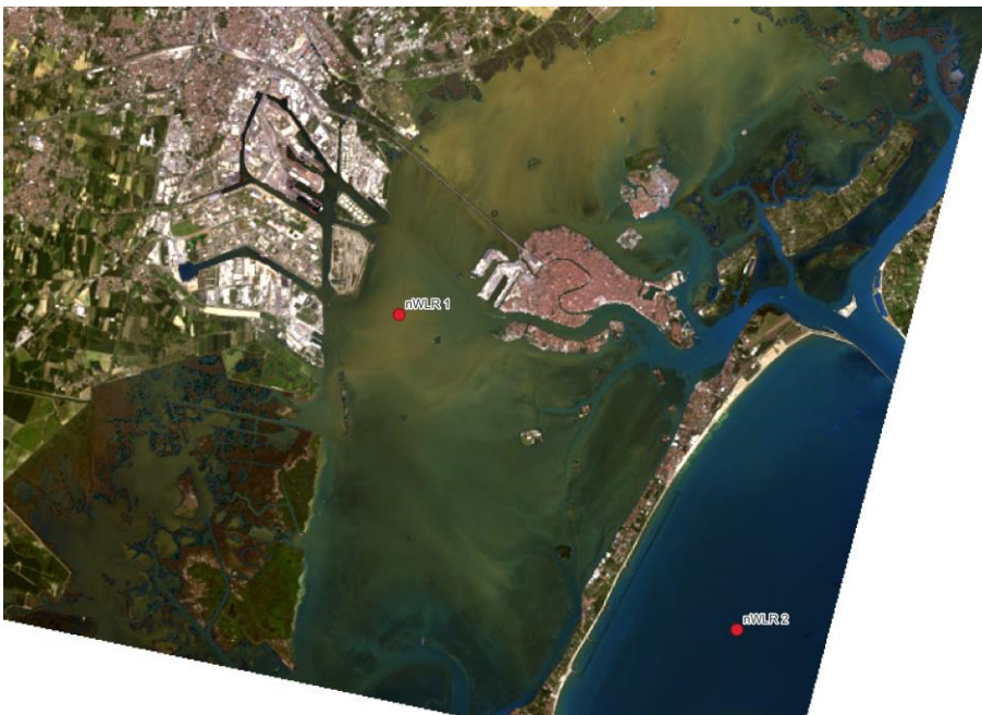
Figure 7-40 Normalized Water Leaving Reflectance of scene-ID 86285; Wavelengths for RGB: 611.02nm – 550.69nm – 463.73nm
