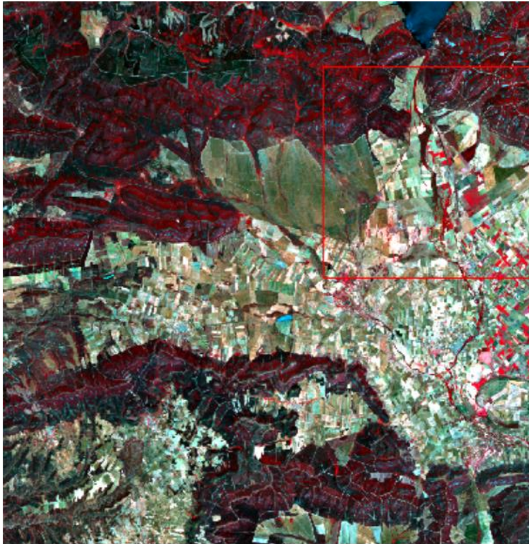
Figure 7-40 Interactive ATCOR processed BOA_ref of scene DT79739 Tile 20 (CIR, bands 75-45-28); note the image is still in sensor geometry.
